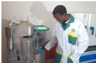
A masters in Chemistry student using a freeze dryer for optimum production cellulose
