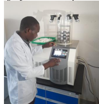
A masters in Chemistry student using a freeze dryer for optimum production cellulose
