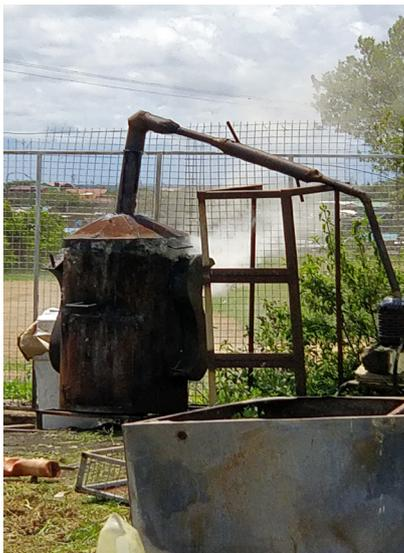
Biomass carbonizing unit in use, with a 90% biomass to bio char conversion efficiency.
