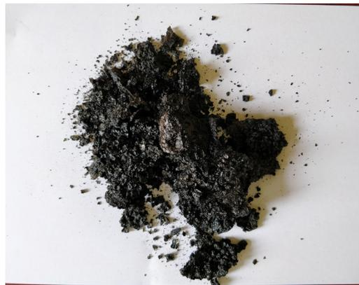
Bio Tar prepared from trash used to make bio char briquettes.
