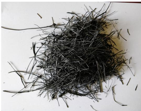
Grass Char prepared from trash and cut grass used to make bio char briquettes.
